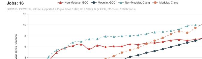
Immediately we can see that the non-modular builds roughly half in clock time matching the doubling of the available parallelism. And are now very close to the performance of GCC modular builds. What is striking is that the modular builds don't substantially change from the 8 parallel job case. And while before modular builds where faster at all depths now the non-modular builds have caught up at the highest depth of this test.
