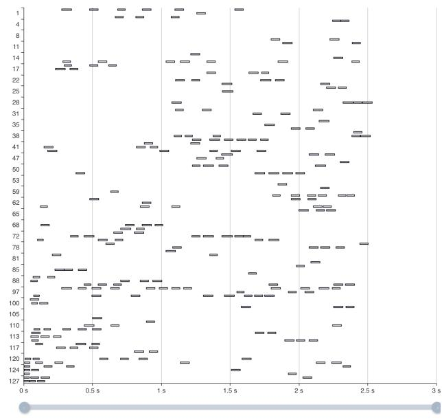
We can see above one key observation, there is a lot of unused CPU time during the overall build execution. This would be due to tasks needing to wait for the needed dependent tasks to complete. Below is the equivalent non-modular build.
